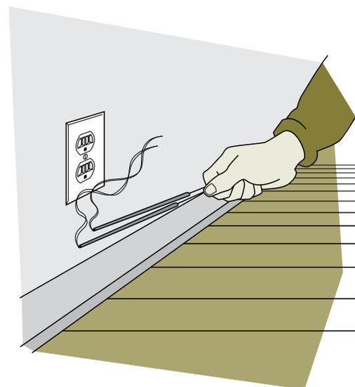
**Figure 4-2** Endroits propices aux fuites d'air
