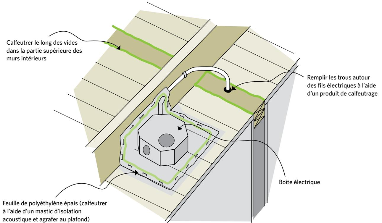
**Figure 5-8** Sceller un luminaire au plafond
