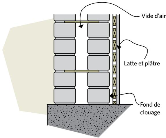
**Figure 7-3** Construction en blocs de béton, un mur mitoyen et un mur ouvert
